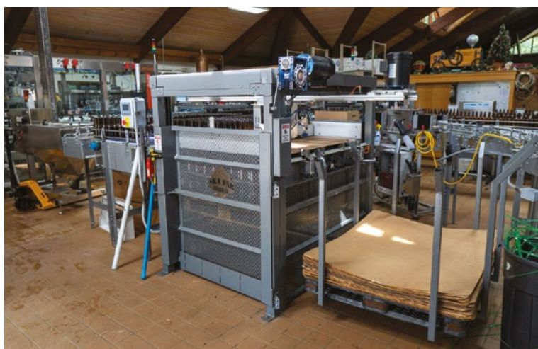
A depalletiser for glass bottles is seen here at Hamburg Brewing Company, Hamburg, New York. (Photo provided courtesy of Ska Fabricating).
